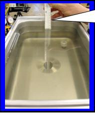
DANGER Moving machinery Fill the Hopper to about 1 inch from the top
